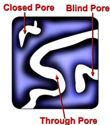
Figure 1: Closed, blind and through pores in materials.
