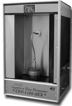
Figure 1. The Microflow Porometer used in this investigation
