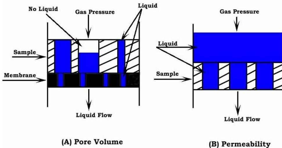
Figure 7: Principle of liquid extrusion porosimetry
