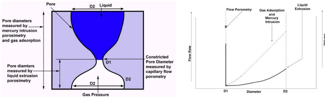
Figure 15: Pore diameter measured by extrusion porosimetry and other techniques.
