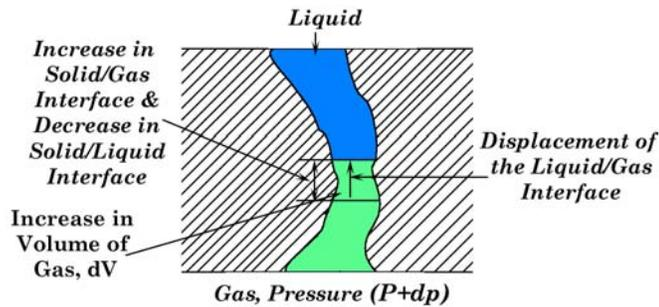
Figure 2: Displacement of wetting liquid in a pore.
