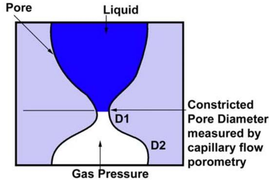
Figure 10: Pore diameter measured by flow porometry.
