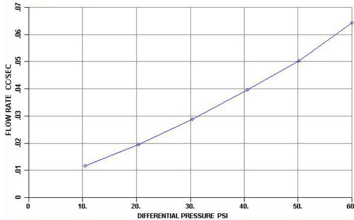
Figure 12. Liquid flow rate of 31% KOH solution through a nonwoven battery separator material
