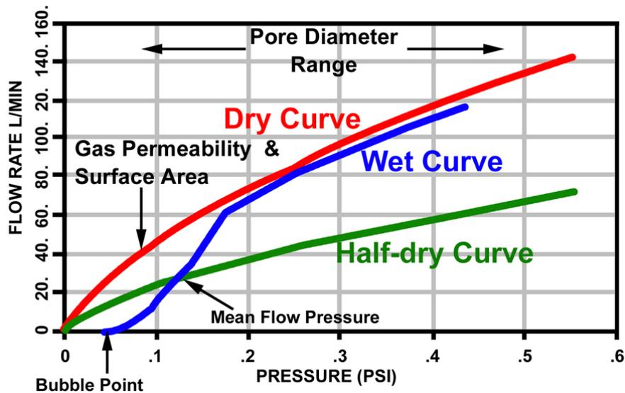
Figure 9: Differential gas pressures and gas flow rates through a sample of nonwoven filter material in wet and dry conditions.
