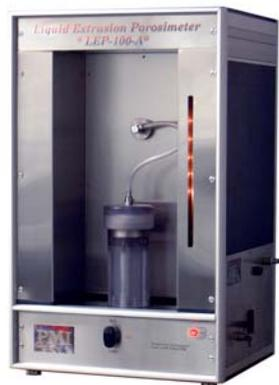
Figure 8. The Liquid Extrusion Porosimeter used in this study.
