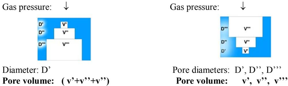
Figure 17. Determination of converging or diverging nature of the pore.
