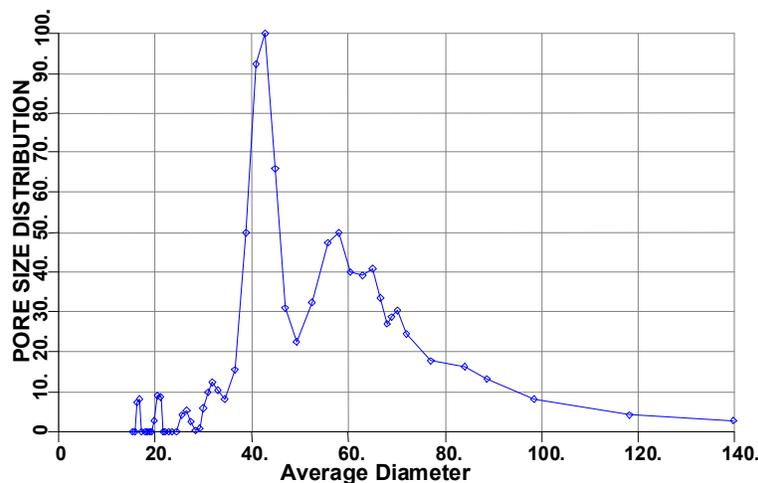
Figure 11: Pore distribution obtained from data in Figure 9.
