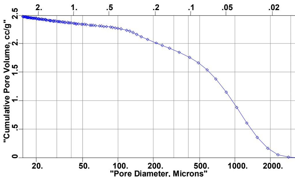
Figure 14. Pore volume measured as a function of pressure
