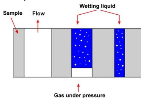
Figure 5. Principle of capillary flow porometry.
