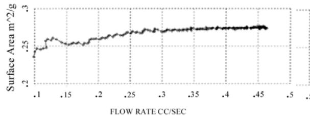
Figure 13. Surface area of a fibrous mat measured as a function of flow rate.
